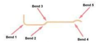
remain as stock. The front vertical slotted portion of the pickup shoe may be bent to limit shoe travel. The rear hook portion of the pickup shoe may be bent to limit shoe travel and adjust shoe tension. The chassis' copper pickup retainer may be bent slightly to improve electrical contact.
