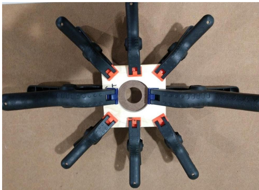
Button 2 – Laminating wood for track call button mount
