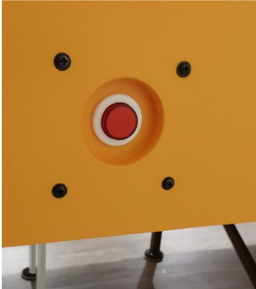
Button 3 – Marshal's track call button mounted to fascia
