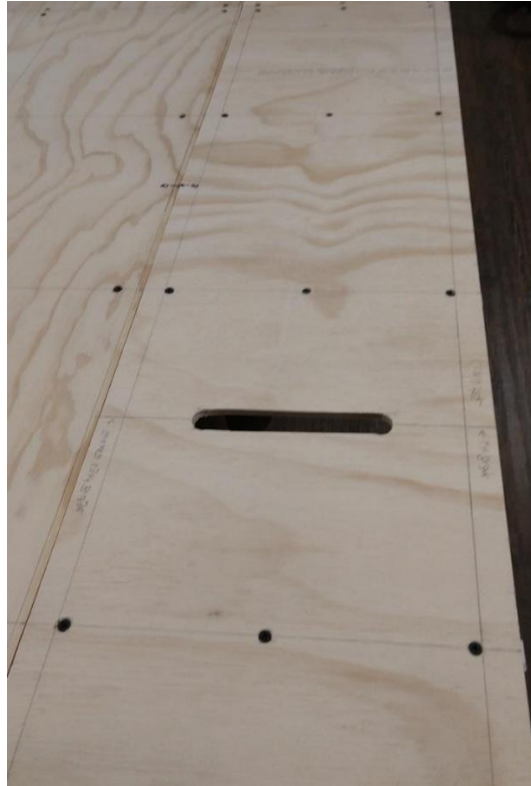
Elevation 9 – Cut Out for LED Track Timing Sensors
