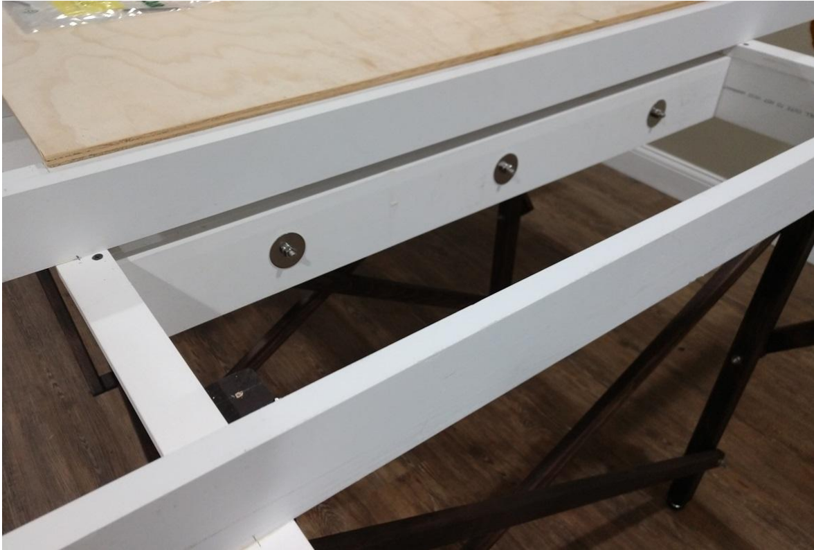
Build 11 – Top View of Benchwork Sections Bolted Together
