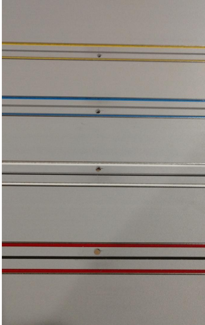
Timing 3 – LED Sensor Holes drilled in Track Section
