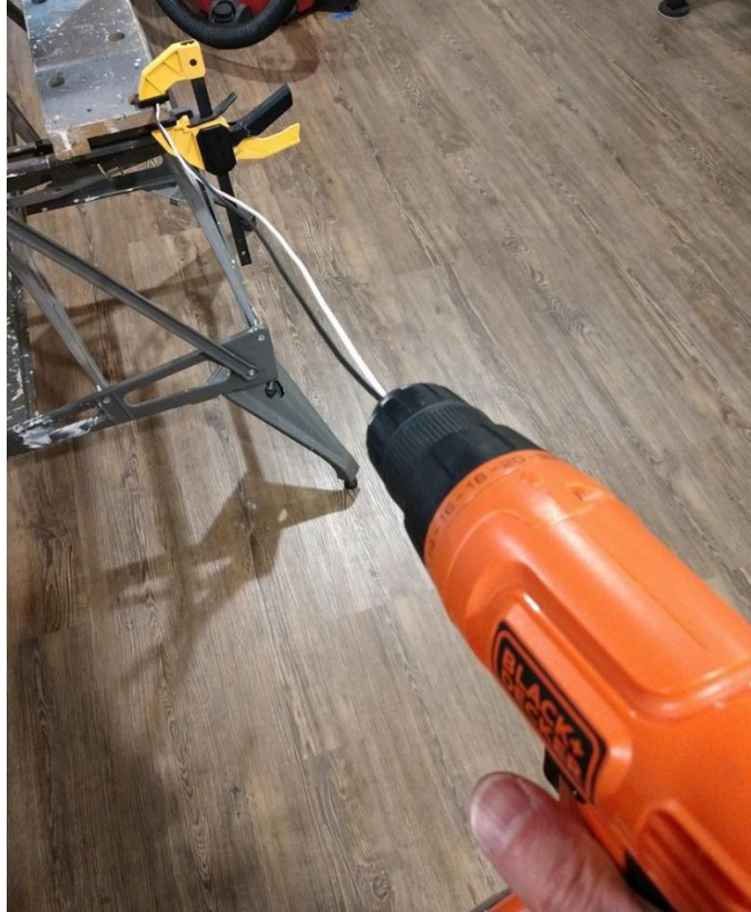
Wiring 7 – Making a cable: wires clamped to stationary bench and other end inserted in to drill chuck
