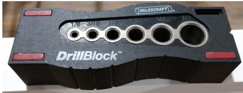
Build 14 – DrillBlock Drilling Jig
