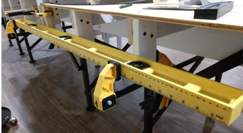
Fascia 3 – Aligning and mounting of fascia supports
