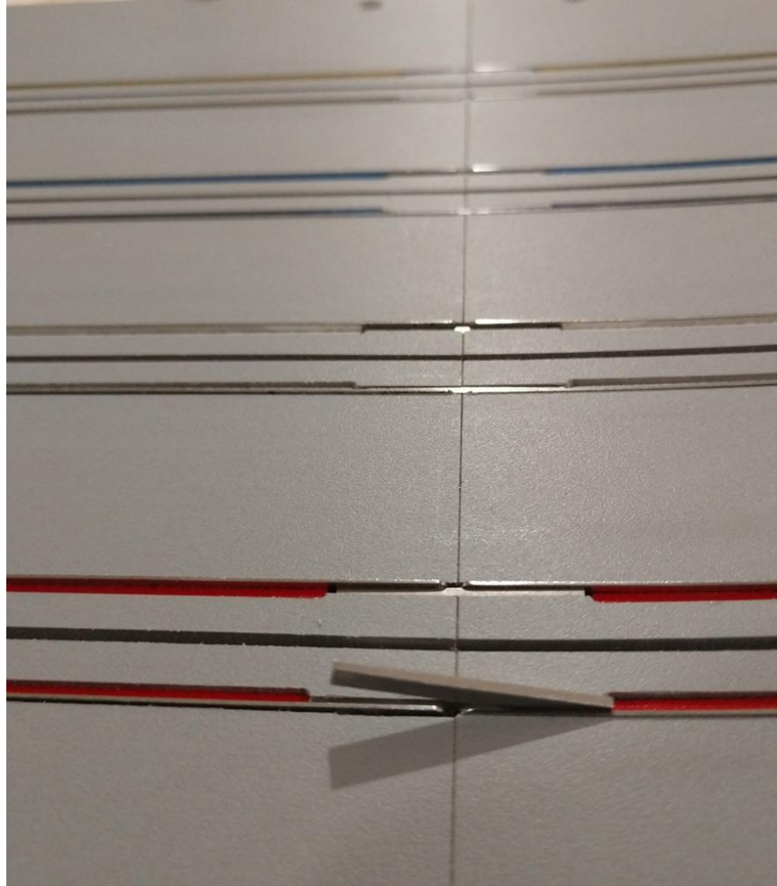
Install 3 – One end of key inserted into one side of track
