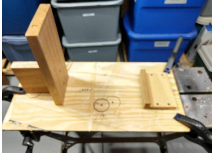
Fascia 15 – Jig for bending hardboard
