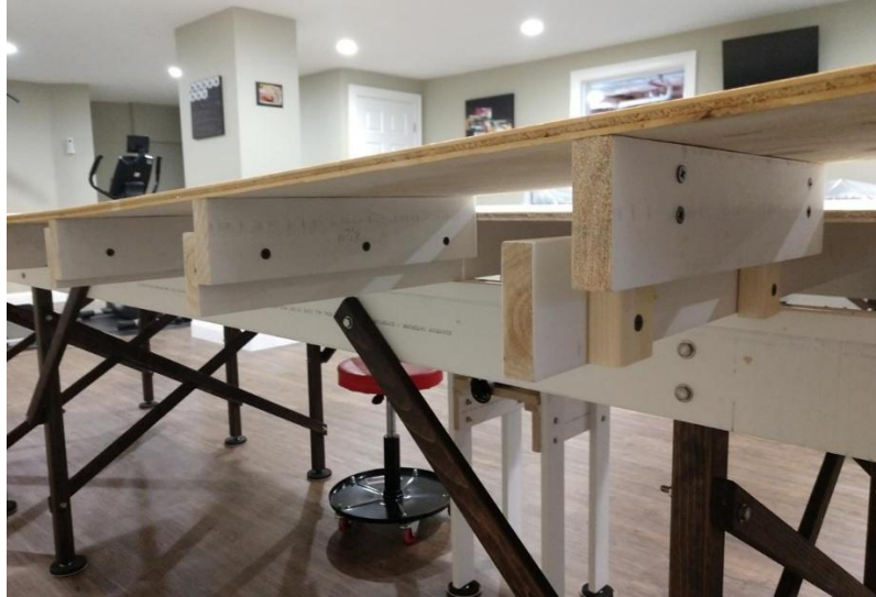
Elevation 3 – Risers Used to Elevate Back Straight
