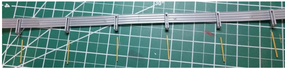
Barriers 3 – Back of modified Armco barrier with cut pieces of 1/16" brass tubing
