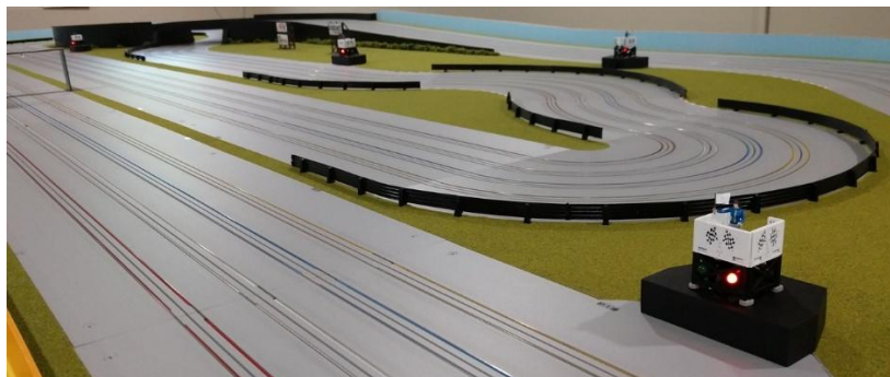
Arduino 1 – Marshal stands with track status LEDs
