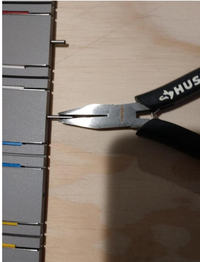
Pin 7 – Inserting Dowel Pins into Track
